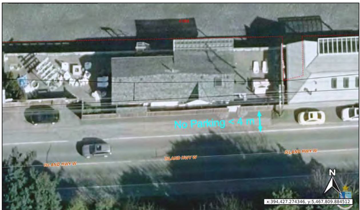
Figure 2.7: Prohibit parking on shoulder less than 4 m wide, Highway 19A
