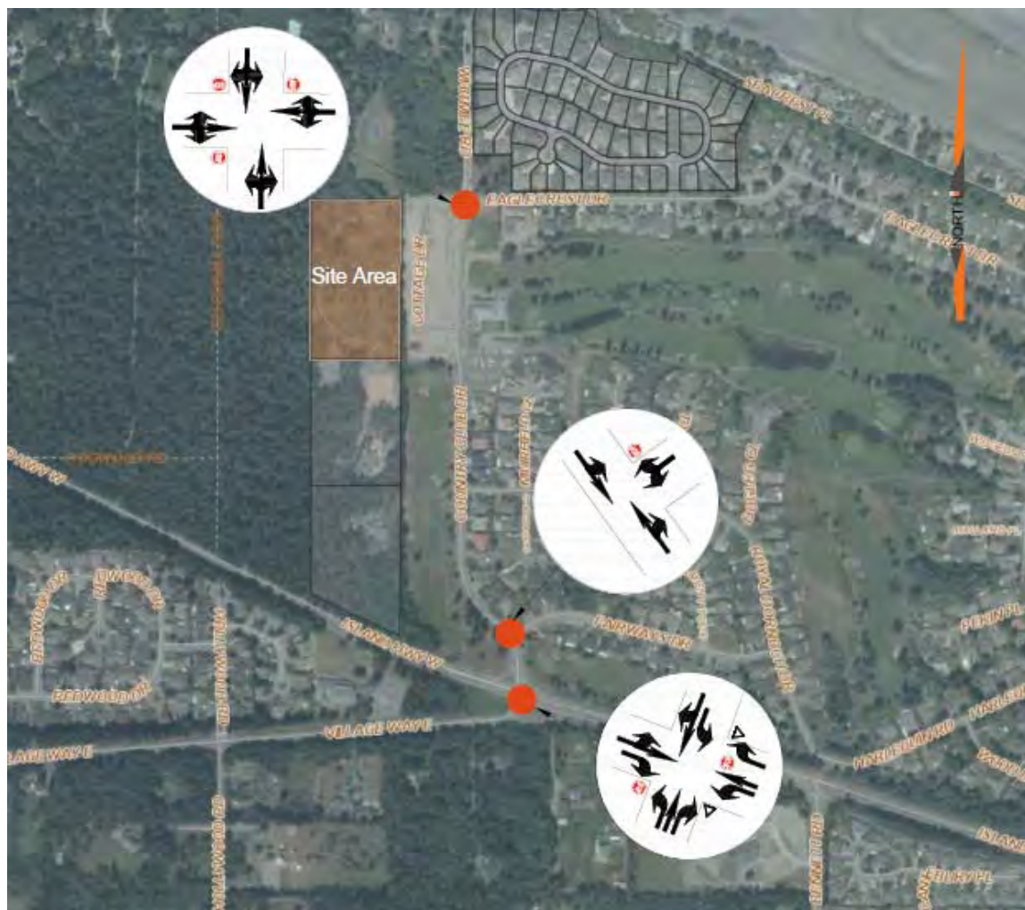
Figure 4: Existing Lane Configuration and Traffic Control
