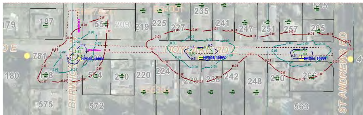
Figure 14: HPS at 55% (potential status prior to upgrade to LED luminaire)
