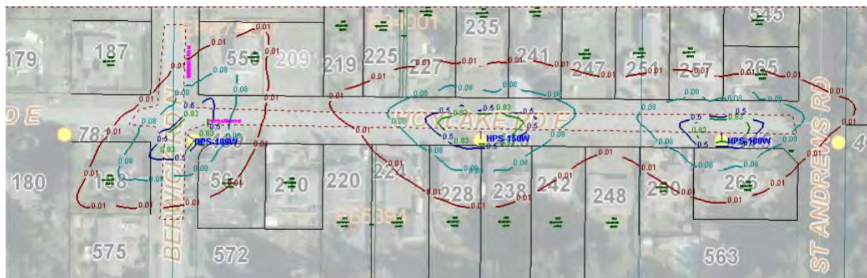
Figure 15 – HPS at 100% (potential status at initial installation of HPS luminaire)
