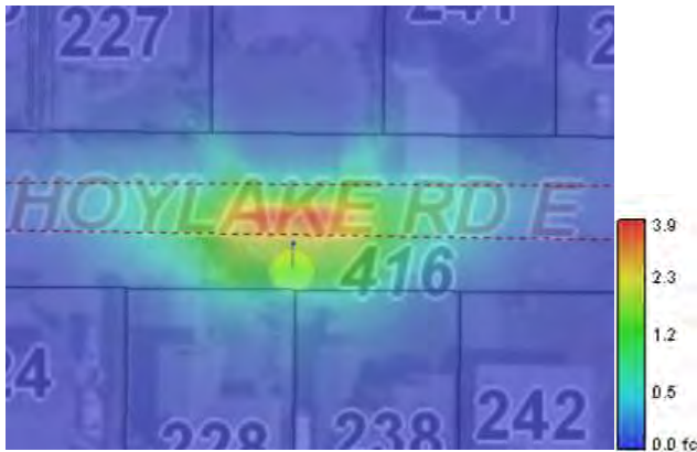
Figure 11: Shaded contour calculation of 150W HPS at 100% (potential status at initial installation of HPS luminaire)
