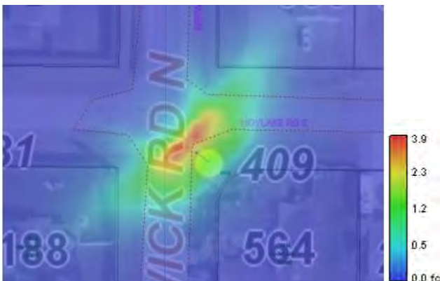
Figure 5: Shaded contour calculation of 100W HPS at 100% (potential status at initial installation of HPS luminaire)
