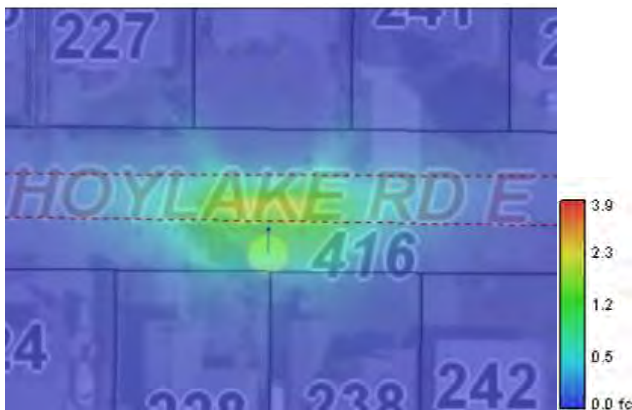
Figure 9: Shaded contour calculation of 150W HPS at 55% (potential status prior to upgrade to LED luminaire)
