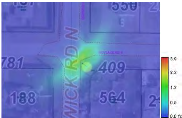
Figure 3: Shaded contour calculation of 100W HPS at 55% (potential status prior to upgrade to LED luminaire)
