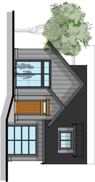
○ East Elevation (Front) Scale = 3/16" = 1'-0"
