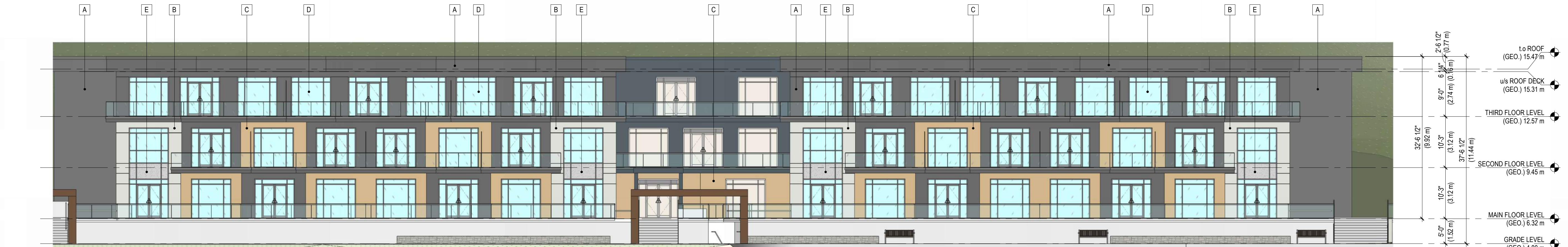
5 NORTH ELEVATION - BUILDING 2 SCALE: 3/32" = 1'-0"
