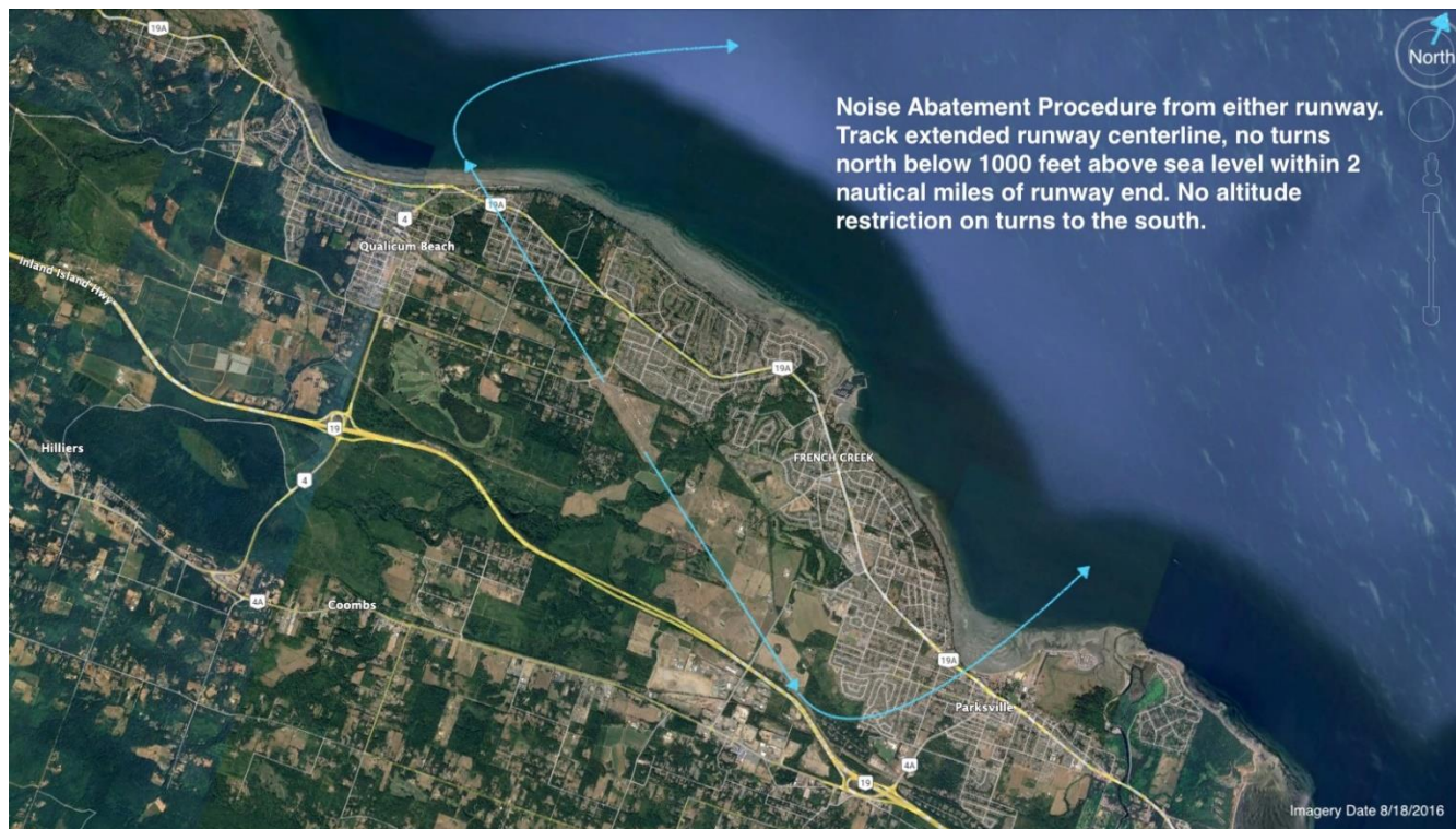
Figure 3 Noise Abatement Procedure (NAP) for turns to the North pursuant to CAR 602.105
